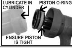
Remove cylinder (8), soak piston o-ring (11) and lubricating washer (13) in NJ Phillips Lubricant.                                                                                                                           |
