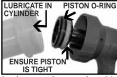
Replace piston o-ring (11) and lubricate liberally.<br>Remove cylinder (8). Hold rear push rod (15), tighten piston (12) firmly using wide blade screwdriver in slot or replace push rod / piston seal ring (if applicable). |
